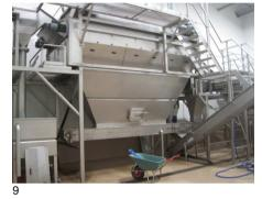
Available in nearly all sizes screw diameters from 500-2500, roller diameters 100 and 150, roller lengths 2000-4000 mm
